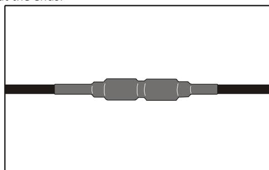
The connectors must be clean and tightened to achieve a good connection
