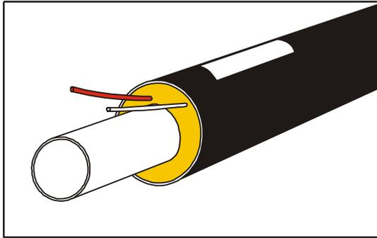
At each joint there must only be one pipe label and it must face upward (12 o'clock position)
