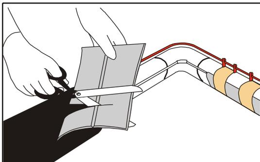
Check that both the steel pipe and the felt are dry during installation.
