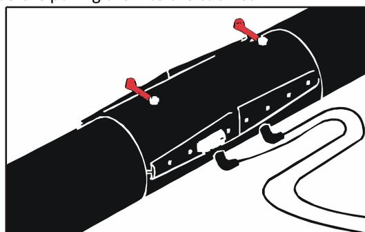
It is recommended to pull the cables between the pipe system and the cabinet through, for example, a PVC-duct. It gives a good protection and facilitates repairs of excavation damages and the like. Measure the connecting point on the pipes in relation to fixed points in the area.
