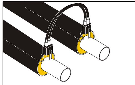
Note! The colour marking, yellow/white, and the colours in the junction box must correspond.
