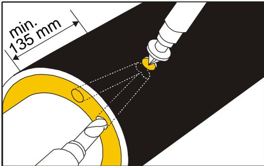
Drill 2 dia. 17 mm holes in to the conical hole.
