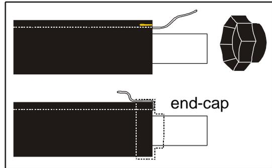
Weld the earth connection on 70 mm from the outer casing end.
