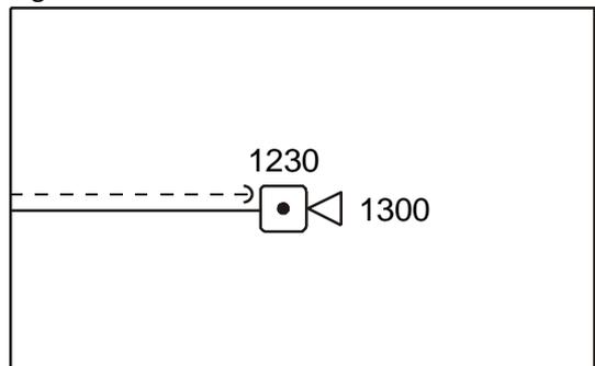
Use long earth connection, part no. 1201 to raise the box above the insulation.
