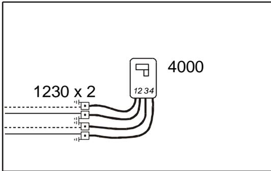
Use long earth connection, part no. 1201 (10 pcs.) so the box is raised above the insulation.
