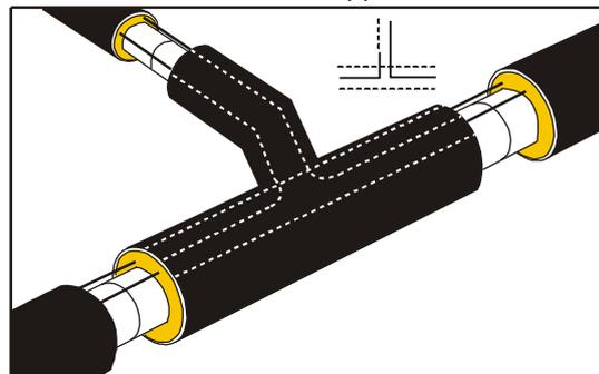
From the illustration it can be seen that the wires from the connected pipe are not used.
