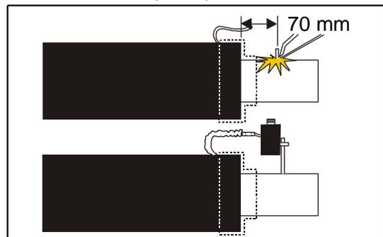
The wire from the connecting/junction box must face towards the outer casing.
