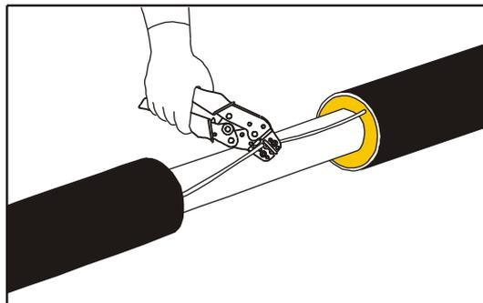
Insert the other wire into the connector and crimp it.
