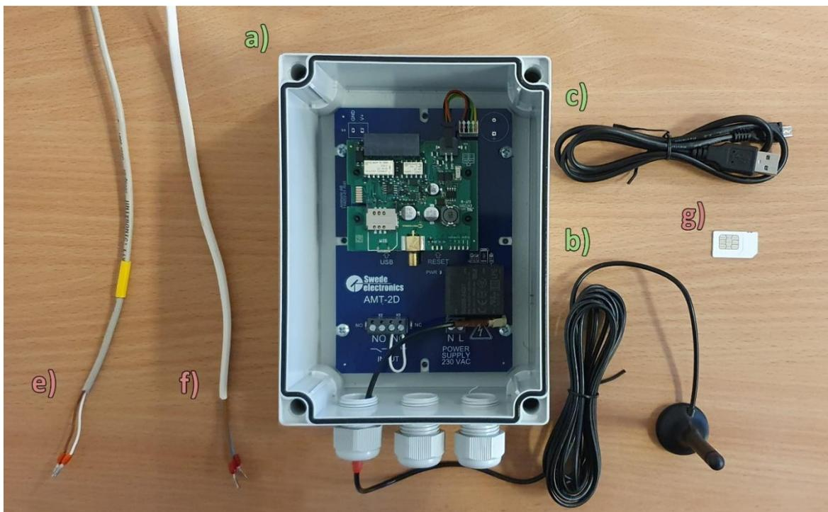
Picture 1 - System components. a), b) and c) are included in the box; e), f) and g) need to be obtained by the user
